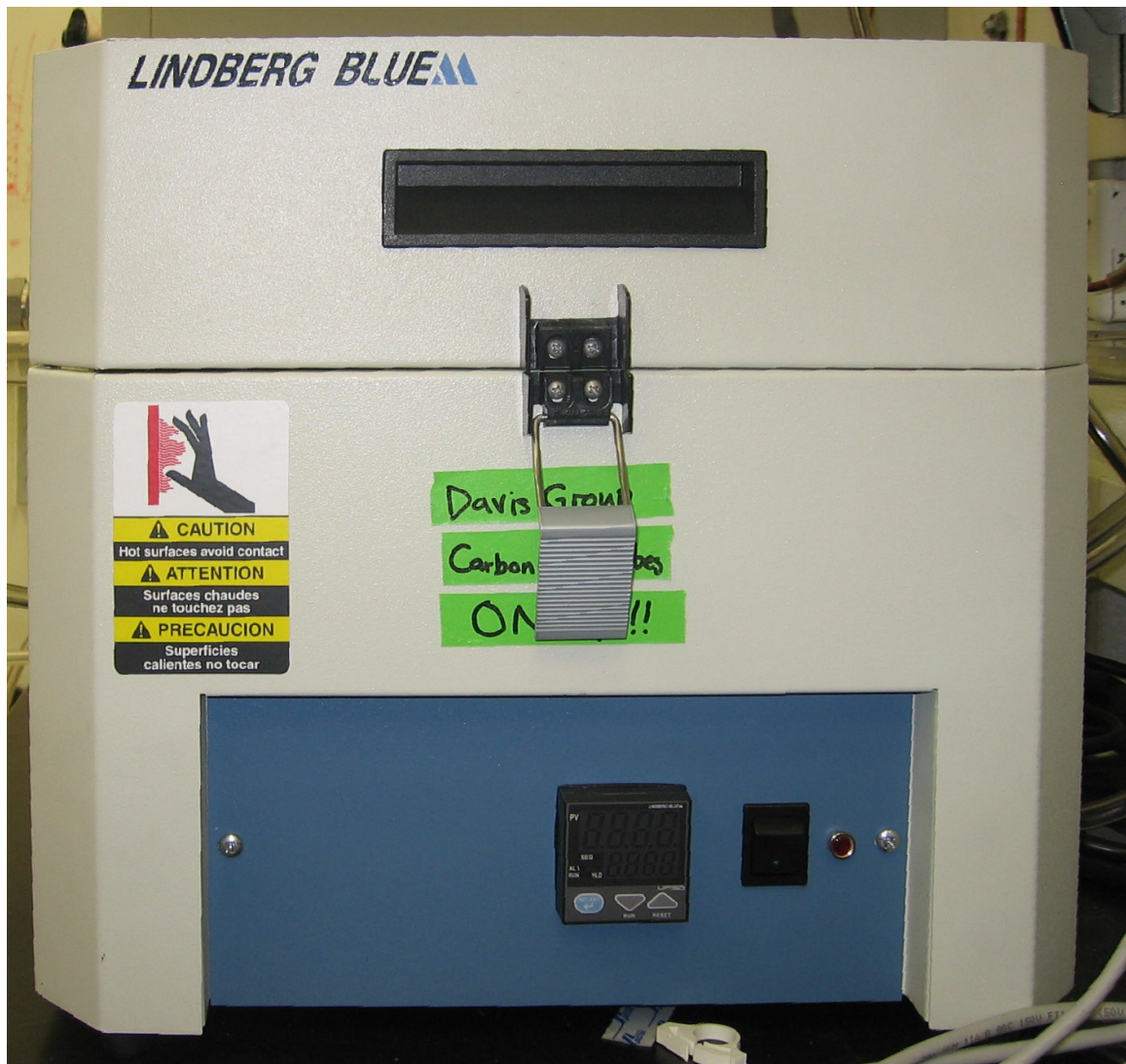
Figure 2.3 Furnace used to perform the argon anneals in.
